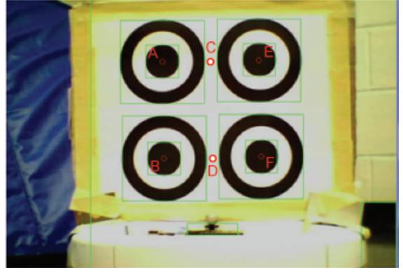
Fig. 2. Blob analysis; detected feature points are marked as red circles
