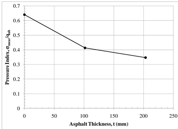
Figure 6. Pressure index as a function of thickness of the asphalt layer.
