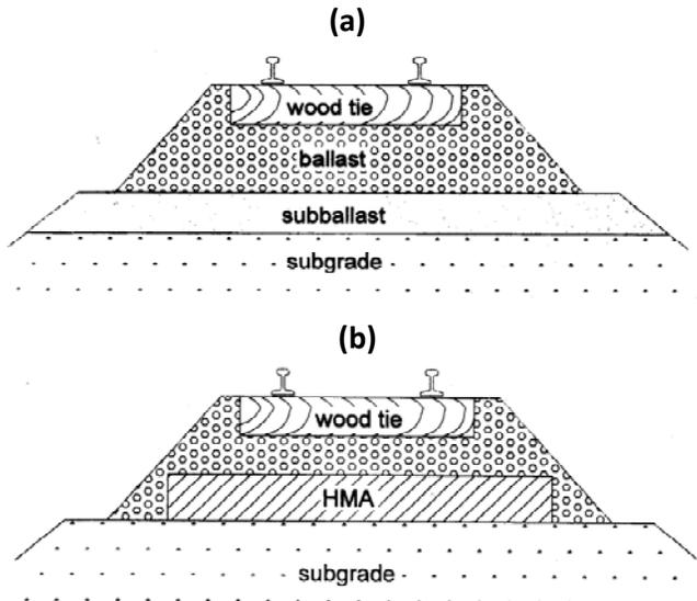
Figure 1. Typical trackbed cross sections: (a) all-granular ballast section; (b) hot mixed asphalt section.
