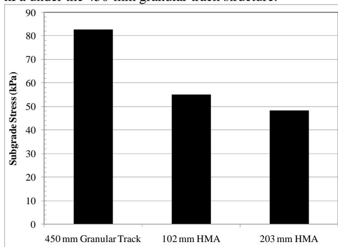
Figure 3. Test Results for Subgrade Stress under 18 metric ton Static Wheel Load.
