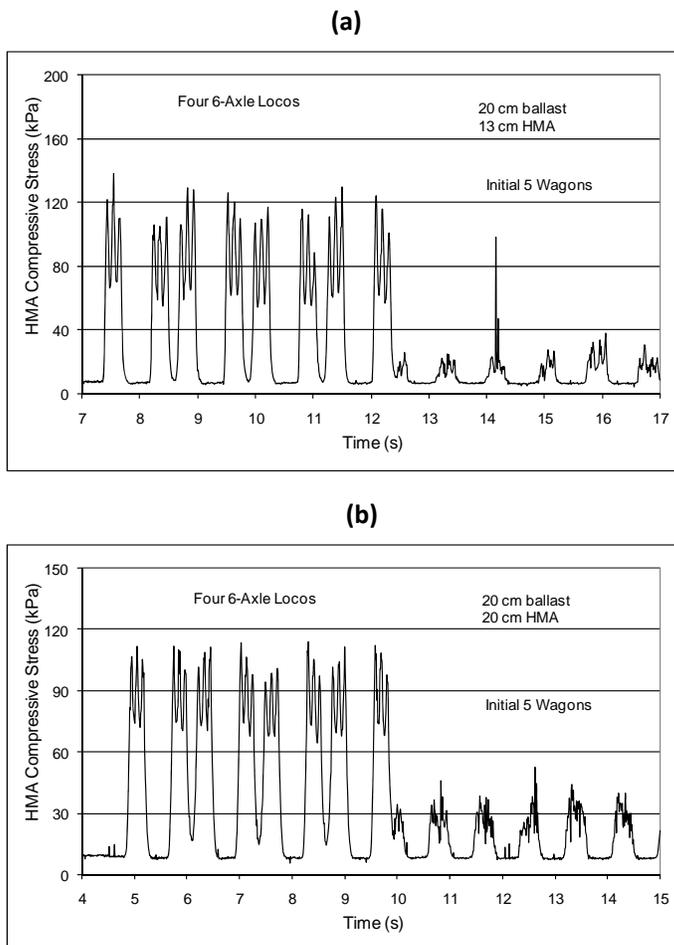
Figure 2. Representative Dynamic Compressive Stress on HMA Layer Measured for Empty Coal Train on CSXT Mainline at Conway, KY: (a) 13 cm HMA Layer; (b) 20 cm HMA layer.
