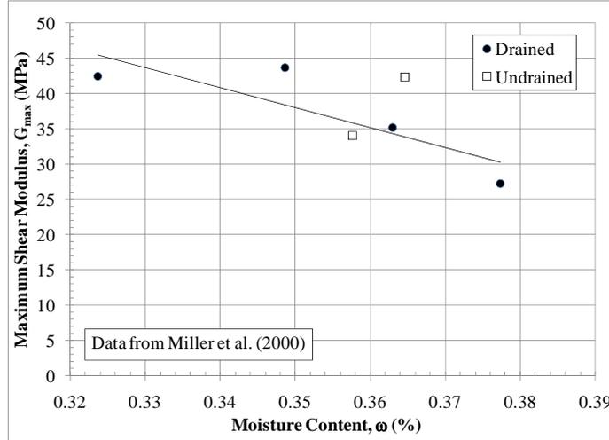
Figure 9. Influence of moisture content of the maximum shear modulus.
