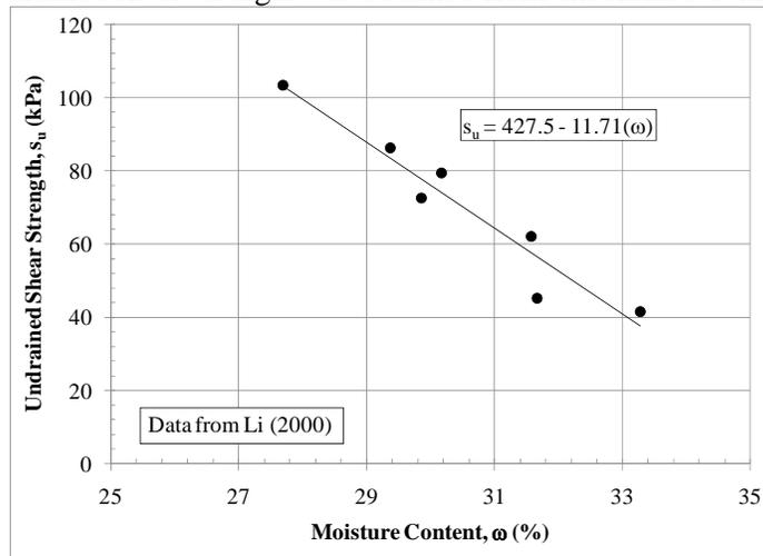
Figure 7. Undrained shear strength as a function of moisture content.
