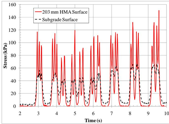
Figure 4. Reduction of Dynamic Stresses from 203 mm HMA Surface to Subgrade Surface under 36 metric ton Axle Cars.
