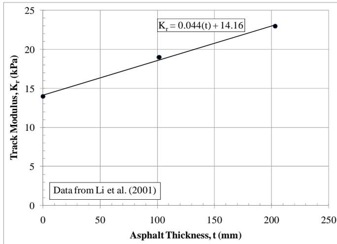
Figure 5. Track modulus as a function of thickness of the asphalt layer.
