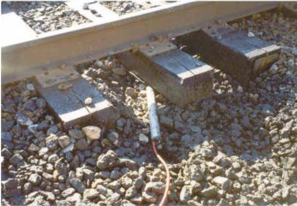
Figure 7. In-Track View of Pressure Cell Testing
