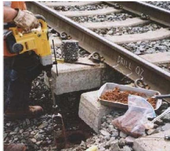
**FIGURE 2 Core drilling operation to obtain asphalt cores and underlying roadbed/subgrade samples.**
