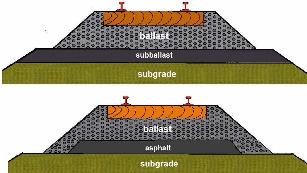
**FIGURE 1 Cross-sectional views of typical all-granular and hot mix asphalt trackbeds.**
