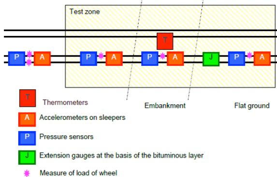
**Figure 3. Instrument layout for SNCF & Colas asphalt trackbed tests (Robinet, 2013).**
