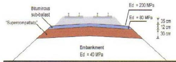
**Figure 4. Cross section of Italian trackbed (Buonanno, 2000).**
