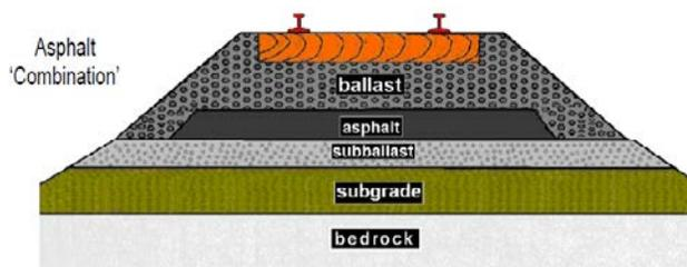
Figure 2b. Asphalt Combination trackbed containing both asphalt and subballast layers.
