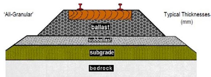
**Figure 1. Classic All-Granular trackbed without asphalt layer.**
