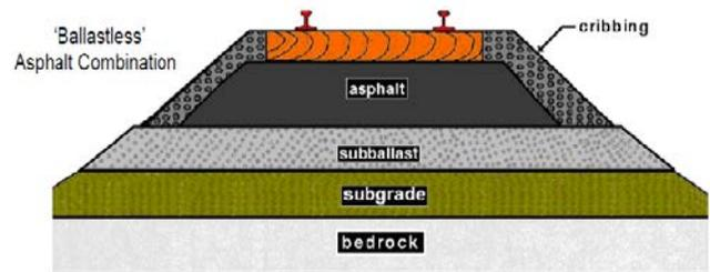
Figure 2c. Ballastless trackbed containing asphalt and subballast layers.
