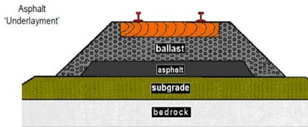
Figure 2a. Asphalt Underlayment trackbed without granular subballast layer.
