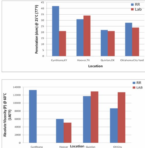
Figure 8. Penetration and absolute viscosity for railroad and laboratory-cured asphalt cores.
