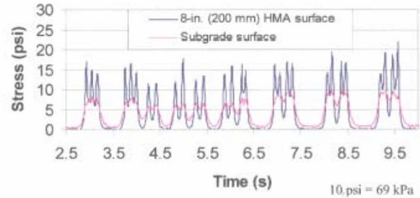
Figure 16. Reduction of dynamic stresses from HMA surface to subgrade surface under 35 MT axle cars.
