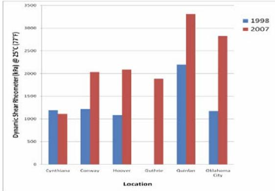
Figure 9. Dynamic shear rheometer values for 1998 and 2007 tests.
