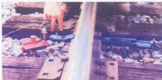
Figure 12b. In-track view of LVDT deflection testing.
