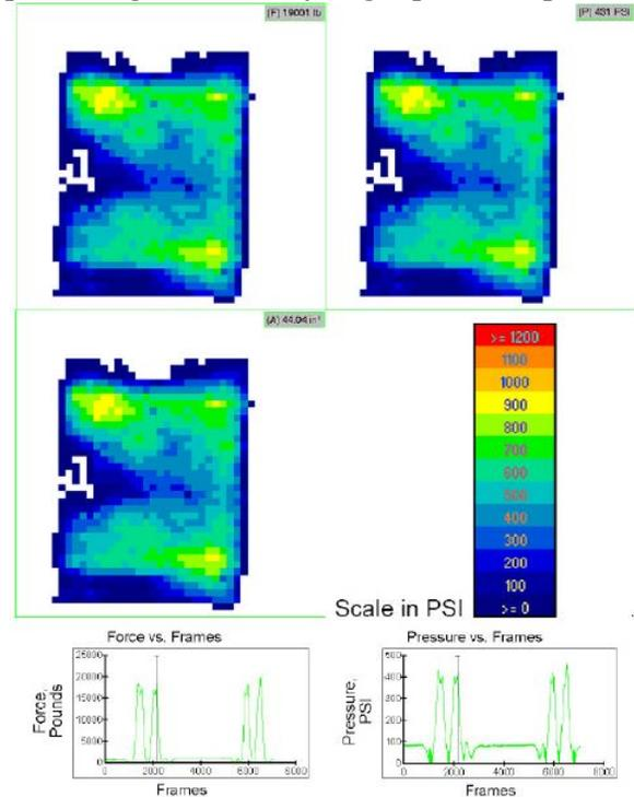
Figure 13. Typical distribution between a machined steel plate and the rail base (Rose and Stith, 2004).
