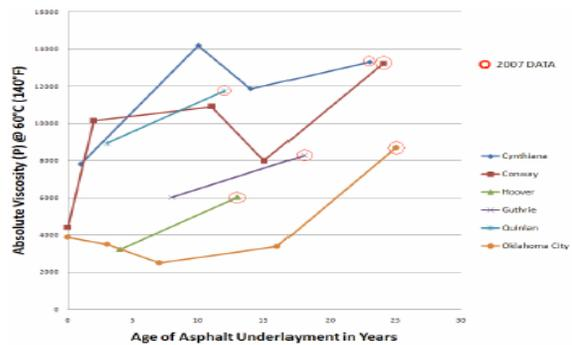
Figure 7. Absolute viscosity versus age of asphalt.
