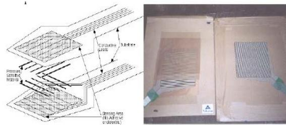
Figure 11a. Basik Tekscan sensor schematic ([www.tekscan.com/technology](http://www.tekscan.com/technology)).
