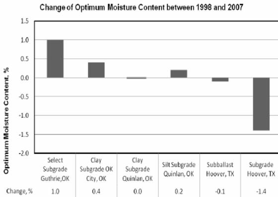
Figure 2. Changes in optimum subgrade moisture.
