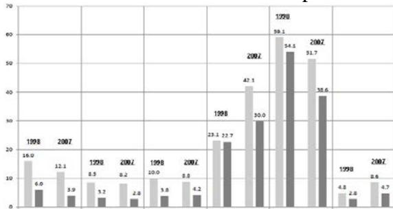
Figure 5. Comparison of 1998 and 2007 unsoaked and soaked CBR test values for the roadbed/subgrade samples.
