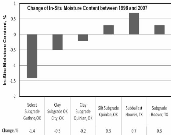
Figure 1. Changes in in-situ subgrade moisture.
