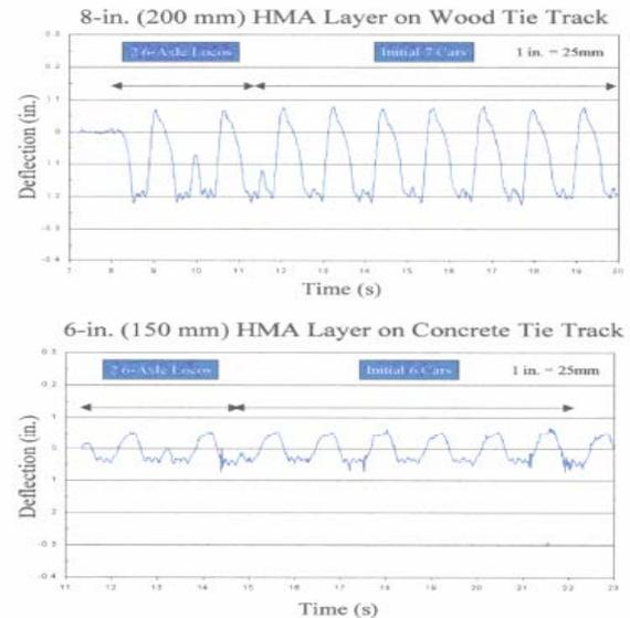
Figure 15. Deflections under loaded coal train.
