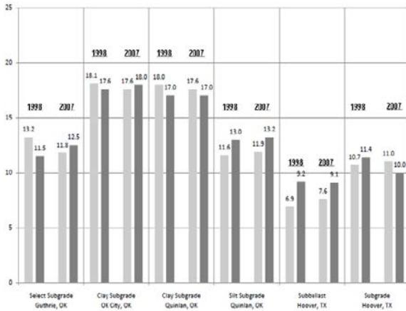
Figure 3. Comparison of 1998 and 2007 measured in-situ moisture contents and optimum moisture contents.
