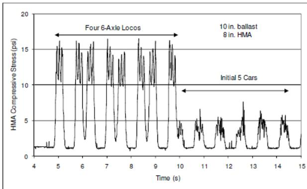
Figure 14. Representative dynamic compressive stress on HMA layer measured for empty coal train.
