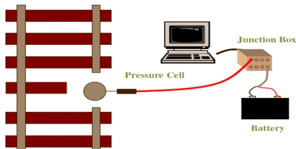
Figure 10. Pressure cell measurement configuration.
