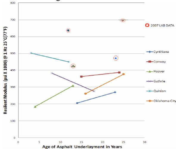
Figure 6. Resilient modulus versus age of asphalt.
