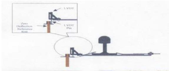
Figure 12a. LVDT measurement configuration.
