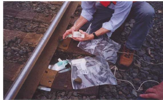
Figure 11b. In-track view of Tekscan pressure distribution system.
