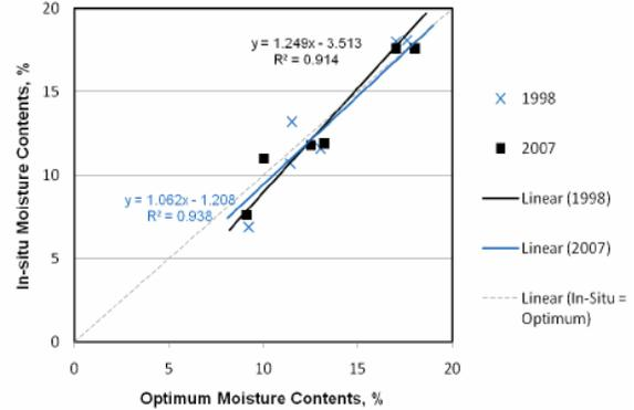
Figure 4. Relationships for roadbed/subgrade in-situ and optimum moisture contents.
