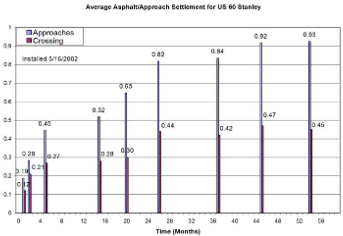
**Figure 6. Top-of-Rail Settlement Data for US 60 Stanley Crossing with Underlayment.**
