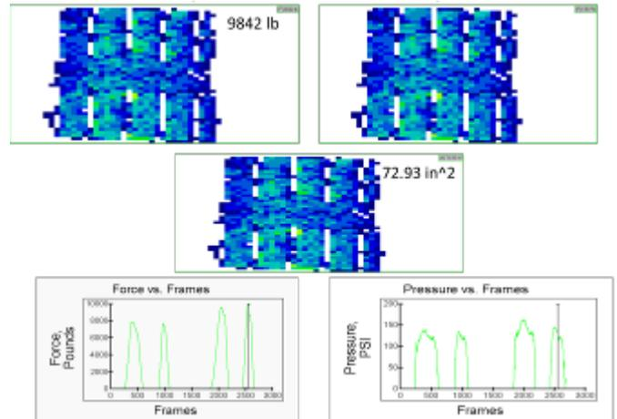
**Figure 5. Imprint of Tractor Rear Tire of Loaded Coal Truck on Concrete Crossing.**
