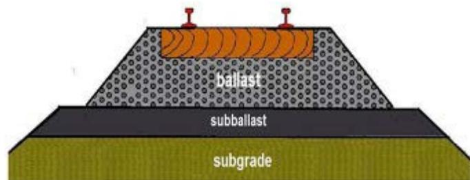
Figure 1a. Typical All-Granular Trackbed.
