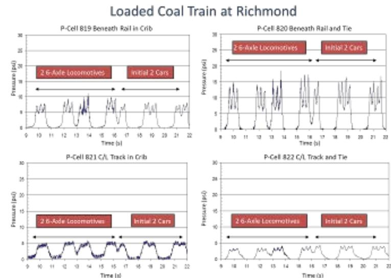
**Figure 3. Typical Pressure on Asphalt in Trackbed for Loaded Coal Train.**
