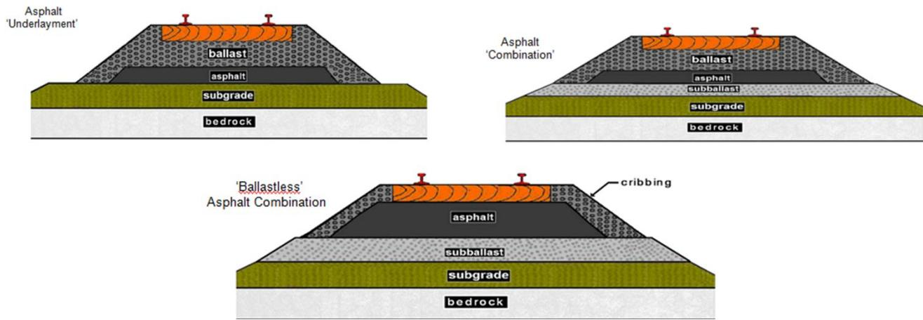
Fig. 1. Various asphalt trackbed designs.
