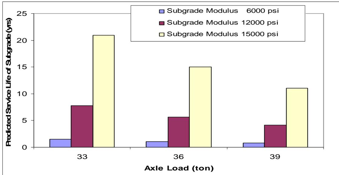
Figure 17: Effect of axle load on the predicted service life of subgrade in ballast trackbed
