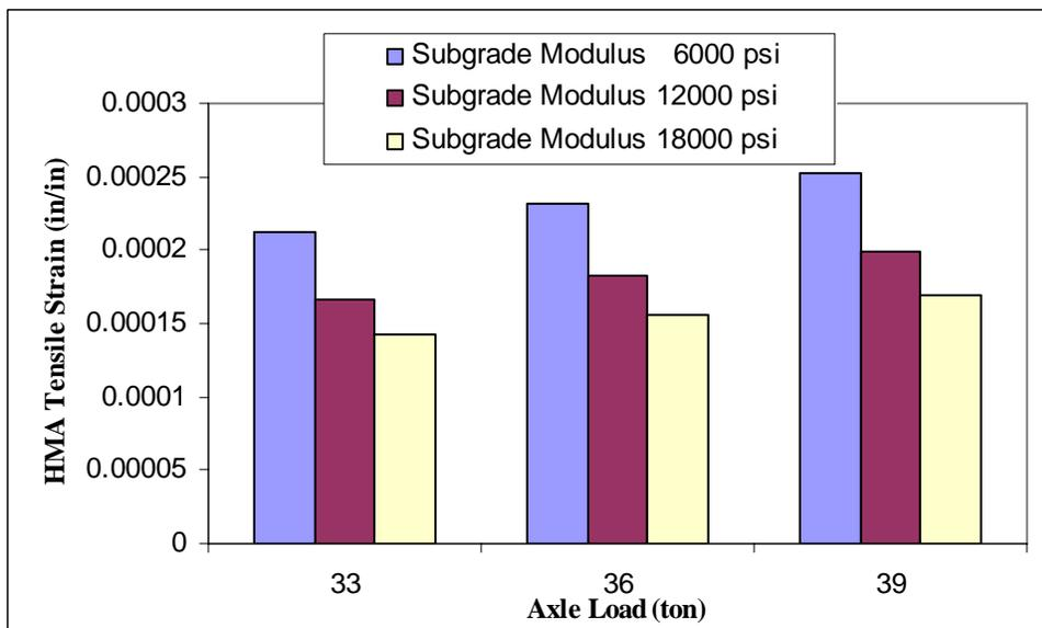
Figure 14: Effect of axle load on the HMA tensile strain in a HMA trackbed
