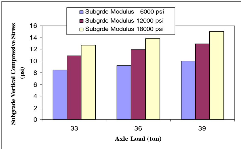
Figure 12: Effect of axle loads on vertical compressive stress on subgrade in HMA trackbed
