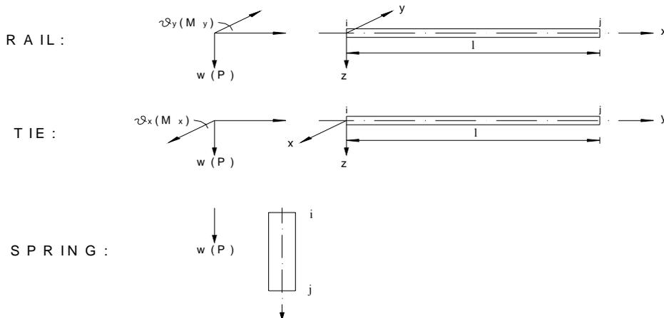
Figure 5: Beam and spring element used in KENTRACK
