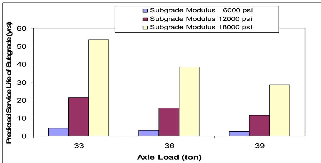
Figure 16: Effect of axle load on the predicted service life of subgrade in HMA trackbed
