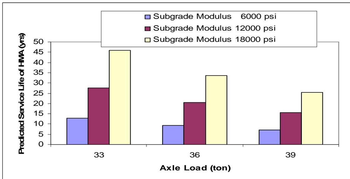
Figure 15: Effect of axle load on the predicted service life of HMA in HMA trackbed
