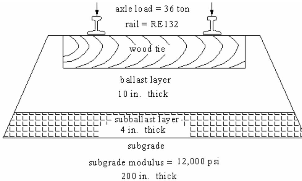
Figure 8 b: All - Granular Track section
