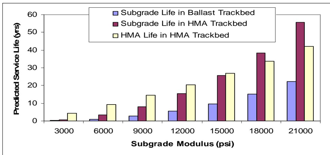
Figure 10: Effect of subgrade modulus on predicted service lives
