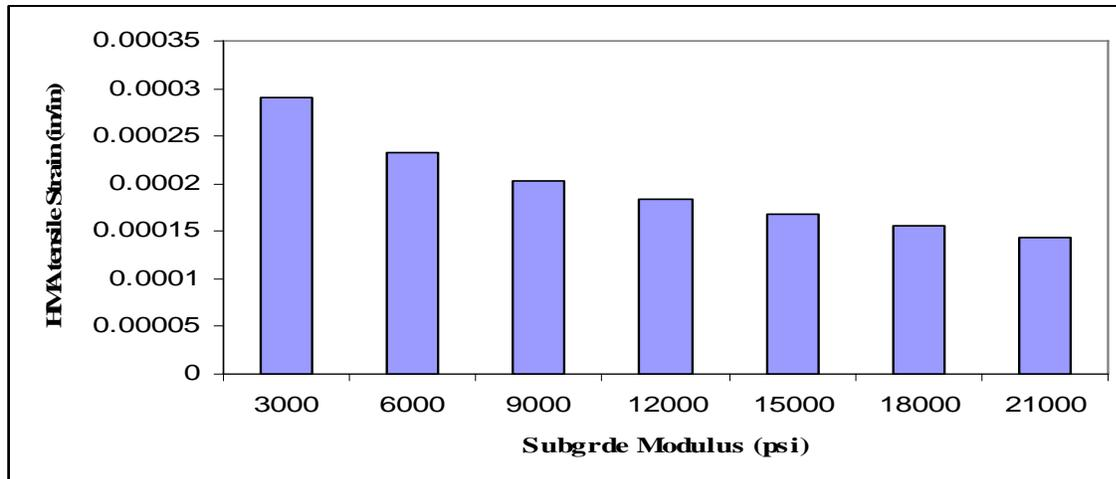
Figure 11: Effect of subgrade modulus on HMA tensile strain
