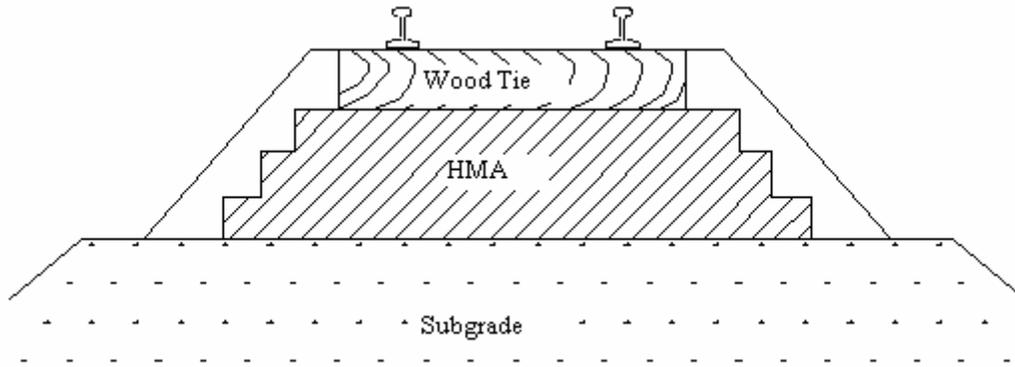
Figure 2: Overlayment Trackbed Design
