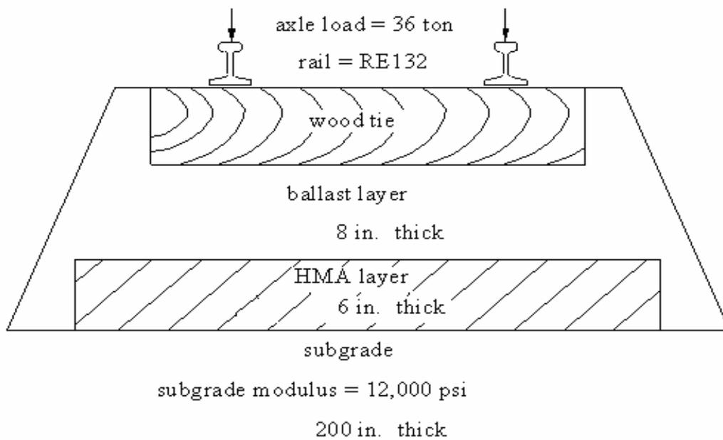
Figure 8 a: HMA track section
