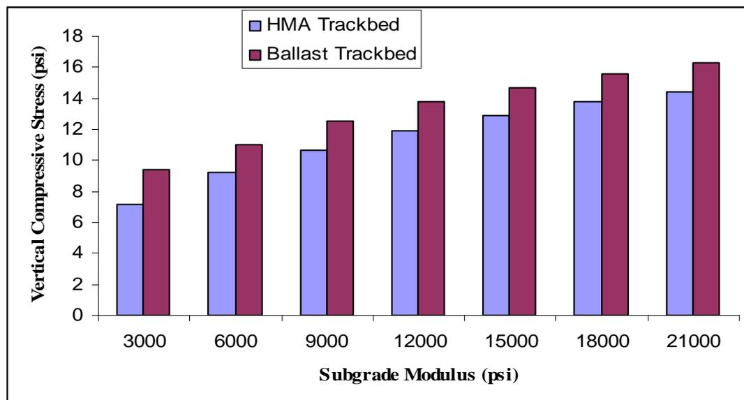
Figure 9: Effect of subgrade modulus on vertical compressive stress
