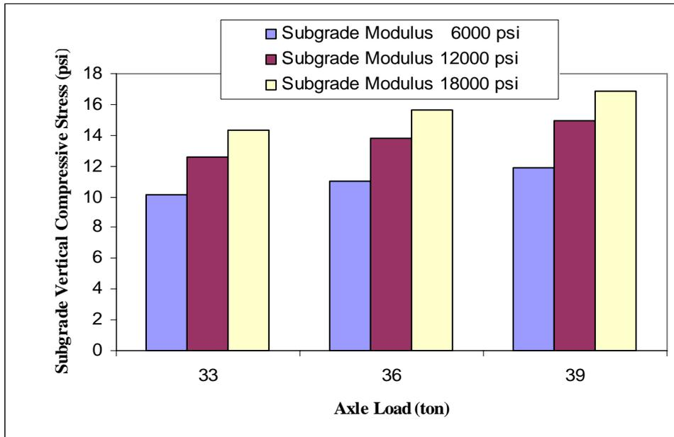
Figure 13: Effect of axle loads on vertical compressive stress on subgrade in ballast trackbed
