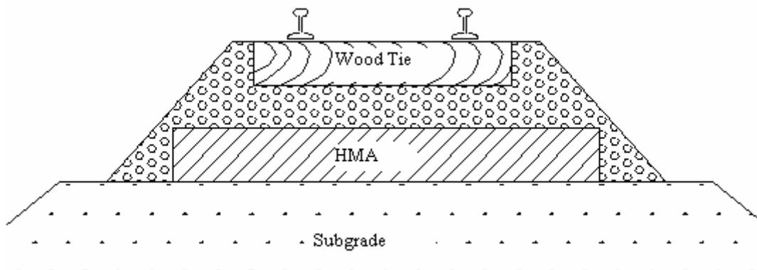
Figure 1: Underlayment Trackbed Design
