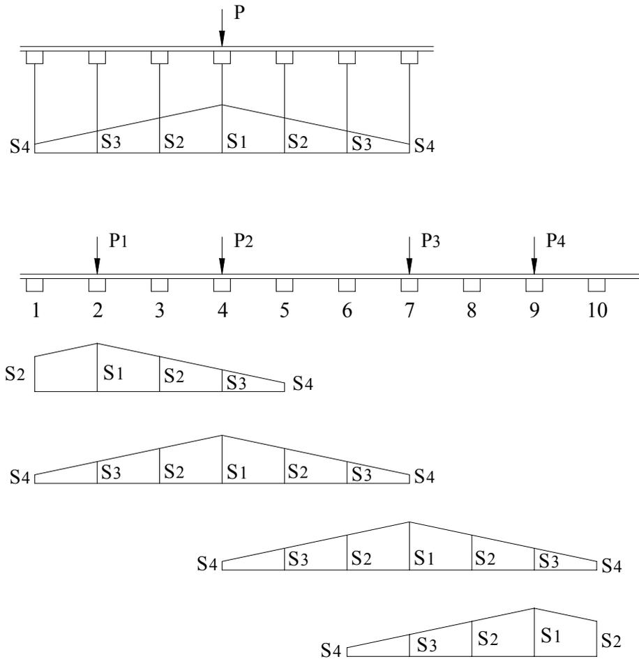
Figure 3: Superposition of multiple loads
