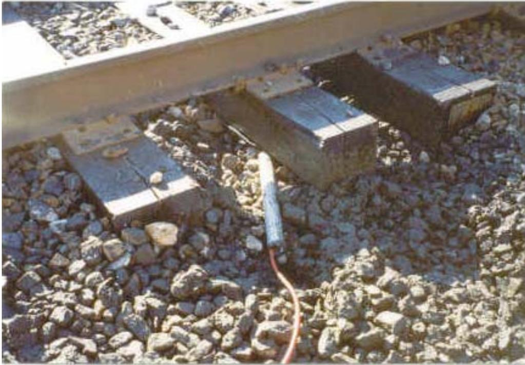
**FIGURE 3b. In-track View of Pressure Cell Testing.**
