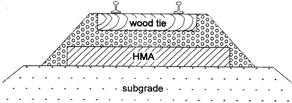
**FIGURE 1b. Typical Hot Mixed Asphalt (Underlayment) Trackbed.**
