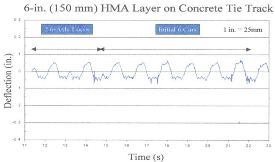
FIGURE 6. Representative Deflections Under Loaded Coal Train.
