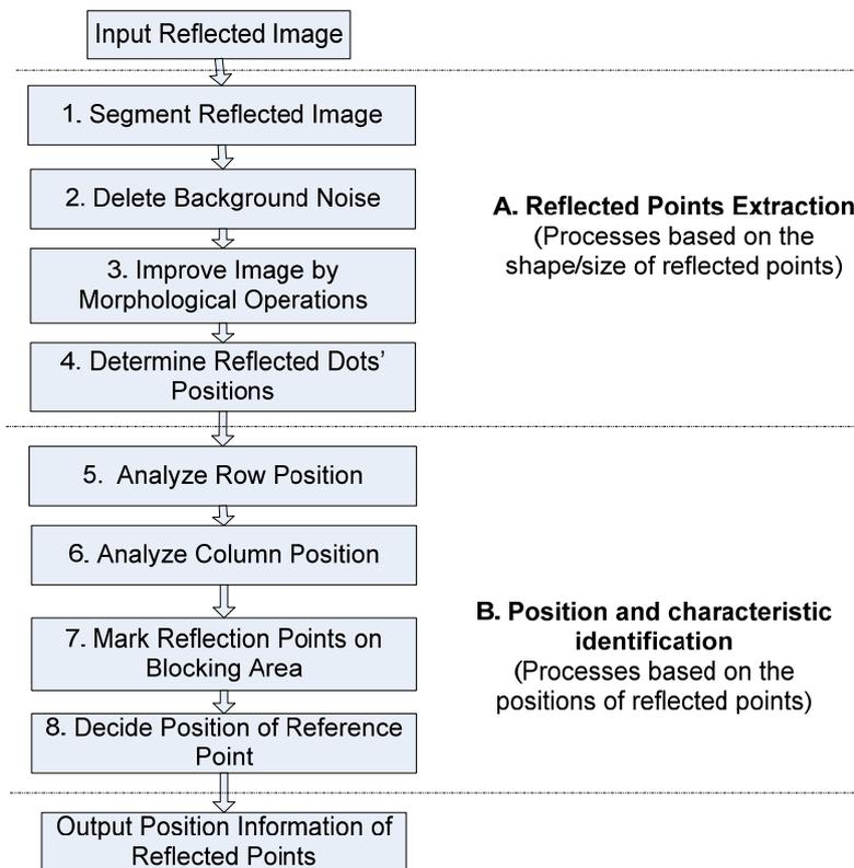
Fig.8 Flowchart for image processing
