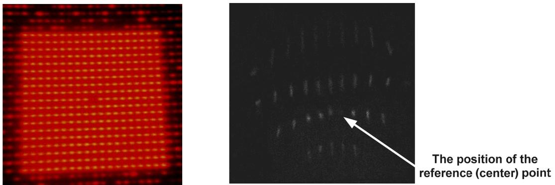
Fig.5 Reference point in (a) projected dot matrix and (b) reflected image
