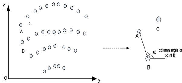
Fig.19 Column angle illustration
