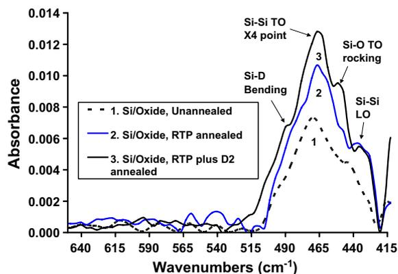
Fig. 1. FTIR spectra of  $\text{Si}/\text{SiO}_2$  samples (23 nm oxide) based on  $n^+$  wafers ( $n = 1 \times 10^{19}\text{ cm}^{-3}$  and  $\rho = 5 \times 10^{-3}\text{ }\Omega\text{ cm}$ ): (1) without any annealing, (2) with RTP annealing ( $1050\text{ }^\circ\text{C}$  in nitrogen for 4 min), and (3) with RTP ( $1050\text{ }^\circ\text{C}$  in nitrogen for 4 min) plus deuterium annealing ( $450\text{ }^\circ\text{C}$  for 30 min).
