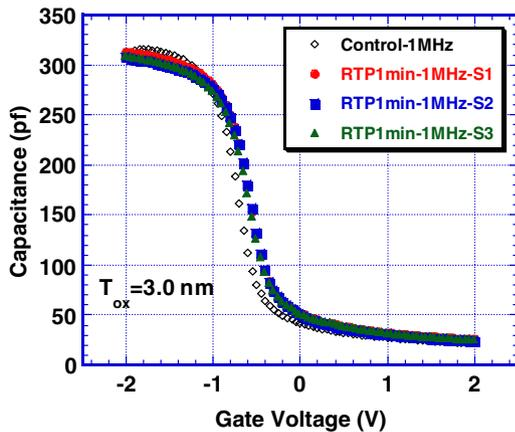
Fig. 12. High-frequency C–V curves of a control sample (before RTP) and samples after RTP at 1050 °C in nitrogen for 1 min with oxide thickness of 3 nm on p-Si ( $4 \times 10^{15} \text{ cm}^{-3}$ ). The samples were finally annealed in 100% D<sub>2</sub> at 450 °C for 30 min.
