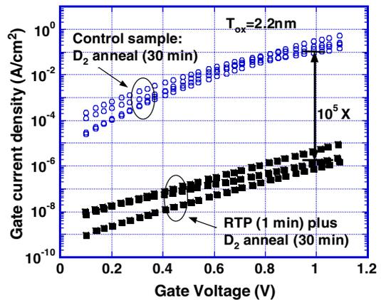
Fig. 11. Gate leakage current density of silicon MOS capacitors with oxide thickness of 2.2 nm on n<sup>+</sup> wafers ( $n = 1 \times 10^{19}$  cm<sup>-3</sup>) with deuterium anneal only (450 °C for 30 min) and with RTP (1050 °C in nitrogen for 1.0 min) plus deuterium anneal (450 °C for 30 min).
