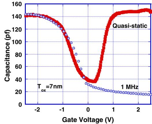
Fig. 13. High-frequency and quasi-static C–V curves of the RTP sample (1050 °C in nitrogen for 1.0 min) with oxide thickness of 7 nm on p-Si ( $4 \times 10^{15} \text{ cm}^{-3}$ ). The sample was finally annealed in 100% D<sub>2</sub> at 450 °C for 30 min.
