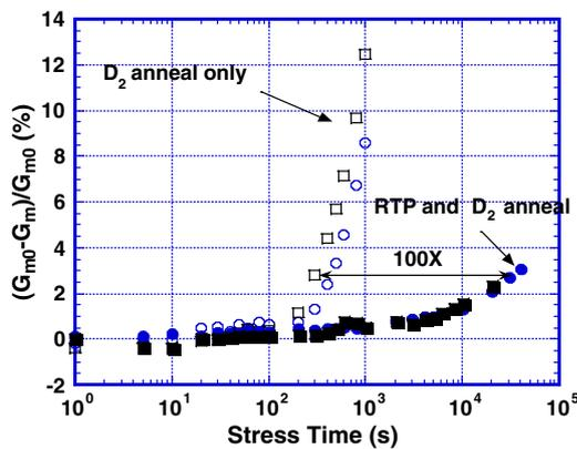
Fig. 5. Comparison of the transconductance degradation of a MOS transistor processed in deuterium only with that processed in RTP plus deuterium anneal. The devices ( $L = 2 \mu\text{m}$ ,  $W = 150 \mu\text{m}$ , and  $T_{\text{ox}} \approx 20 \text{ nm}$ ) were stressed at  $V_G = 5 \text{ V}$  and  $V_D = 12 \text{ V}$ .
