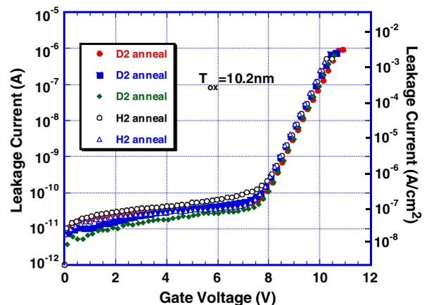
Fig. 7. Gate leakage currents of silicon MOS capacitors with oxide thickness of 10.2 nm and area of  $4.24 \times 10^{-4} \text{ cm}^2$  annealed in hydrogen and deuterium (450  $^{\circ}\text{C}$  for 30 min).
